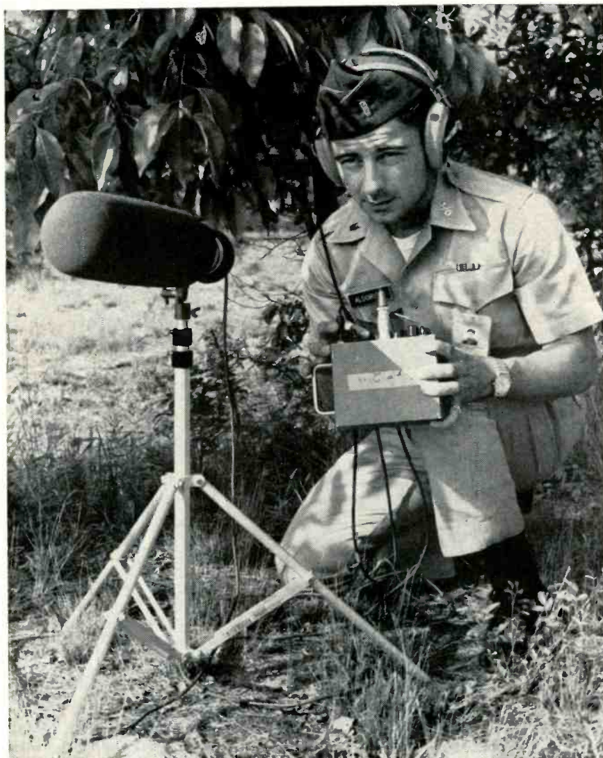
An acoustical telescope, made by Electro-Voice, Inc. for commercial use, is being tested by the Special Forces. The main problem so far is its inability to filter out unwanted sounds.
