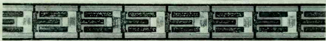
Beam leads provide a large handle for tiny transistor chips (the smallest visible squares). Such strips could be fed to automatic bonding machines.
