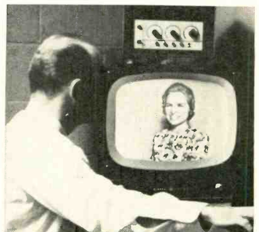
Another example of the General Electric Co low light level tv in action. The faint ambient light in the photo at left was necessary to take the picture. The shot above shows how the model looks on the monitor.
