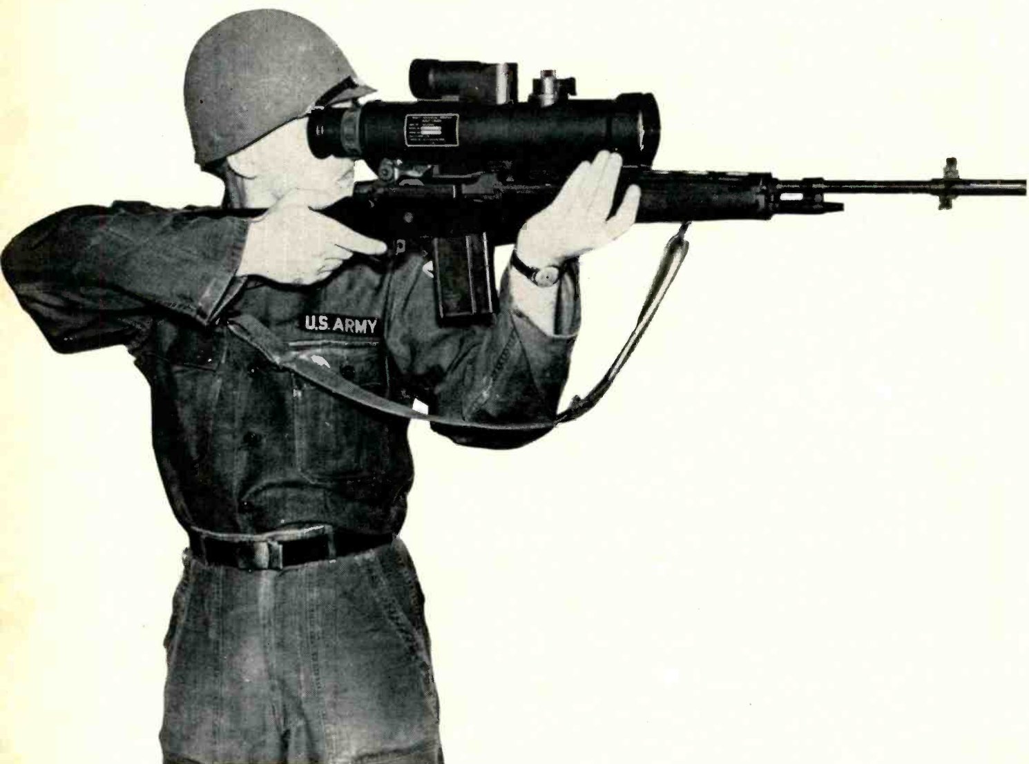
Gun mounted image intensifiers help soldiers to see in the dark without revealing their presence.
