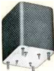
Low frequency band pass filter. Designed for 2.5 cps center frequency. At 2 to 3 cps within 3 db. At 1.5 cps and lower, and 4 cps and higher, greater than 30 db. Source and Load 10K ohms. Size: 4 x 4-11/16 x 6". MA MIL case, MIL-F-18327B.
