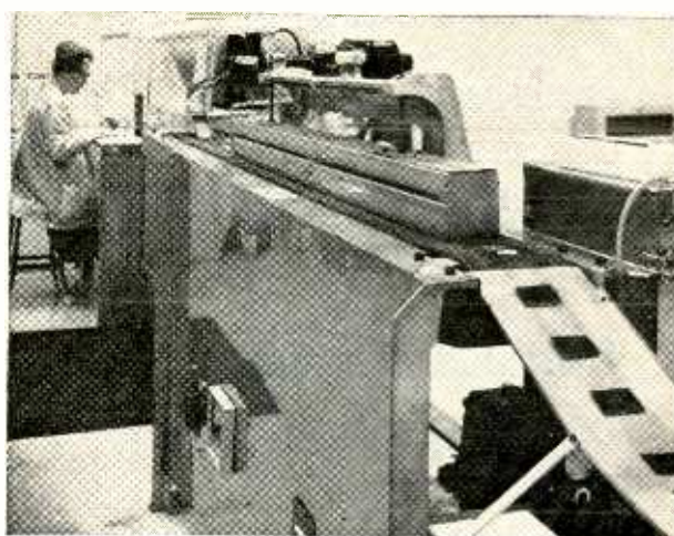
Substrates on their way to the etching station. The tin oxide has just been coated with photoresist.
