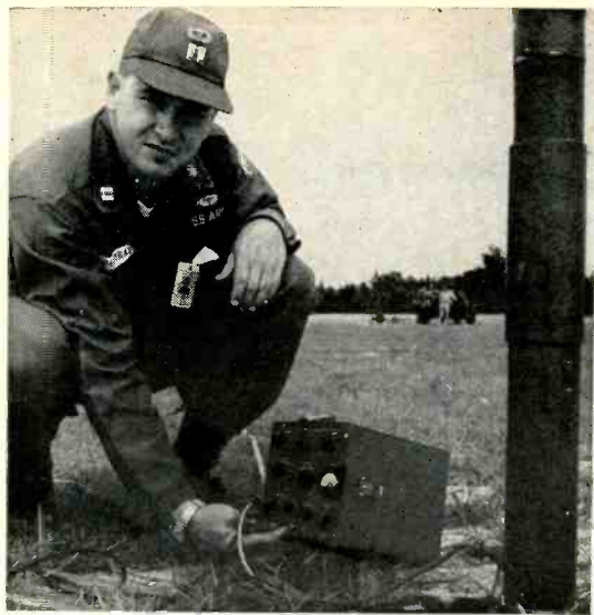
This low-frequency radio beacon for guiding aircraft to a drop zone is the TRN-19, built by Tridea, Inc. It is one of four being tested by the Army.
